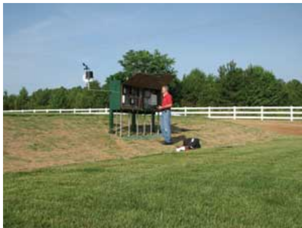
At the turfgrass field lab, Dr. Garry Grabow checks an irrigation controller that is connected to soil moisture sensors.
